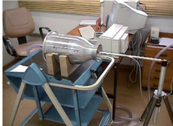
Figure 8: Combustion chamber acoustic testing conducted by Pirk et al. [14]
