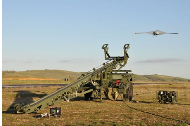
Fig. 6 Hydraulic launcher being used to deploy the RQ-7 Shadow 200[9].
