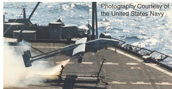
Fig. 8 A Navy RQ-2A firing its rocket booster for deployment on ship [11].
