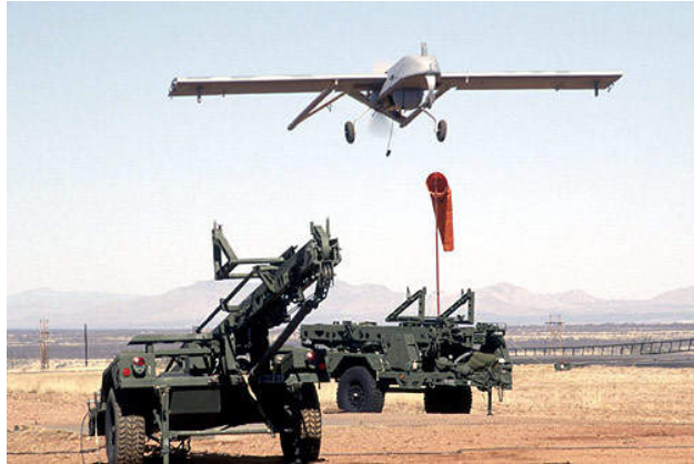
Fig. 21 Hydraulic Launch of an RQ-7 Shadow [33].
