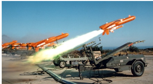
Fig. 15 A RATO Launchpad and Rail Guides the UAV at Launch [22].
