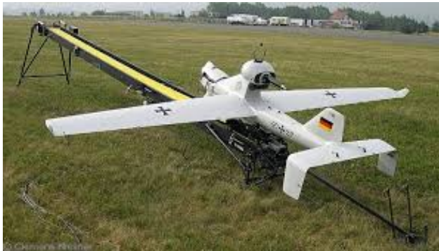
Fig. 4 Example of an elastic launcher used to deploy the LUNA UAV[7].
