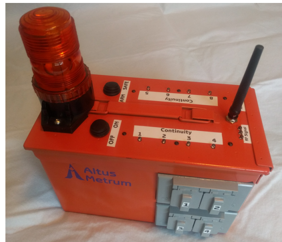
Fig. 17 The Altus Metrum TeleFireEight Controls 8 Launchpads [24].
