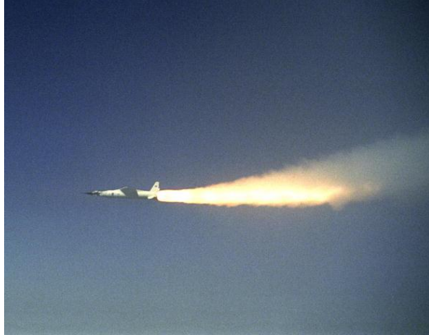
Fig. 9 A modified Pegasus rocket ignites moments after release from the B-52B, beginning the acceleration of the X-43A over the Pacific Ocean [12].
