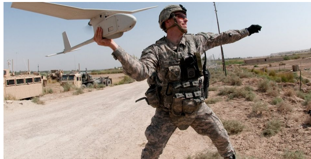
Fig. 19 Hand Launch of an RQ-11 Raven [28].
