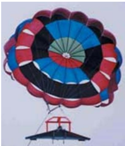
Fig. 2 Example of an exdrone taking off using a parasail [5].
