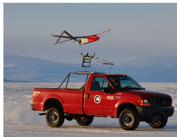
Fig. 3 Example of using an external vehicle to get a UAV up to launch speed [6].
