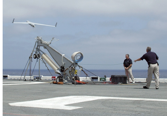
Fig. 5 Example of a pneumatic launcher[8].
