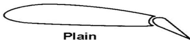
Figure 2.12: Flap configuration for increasing lift (Jacob, 2017)
