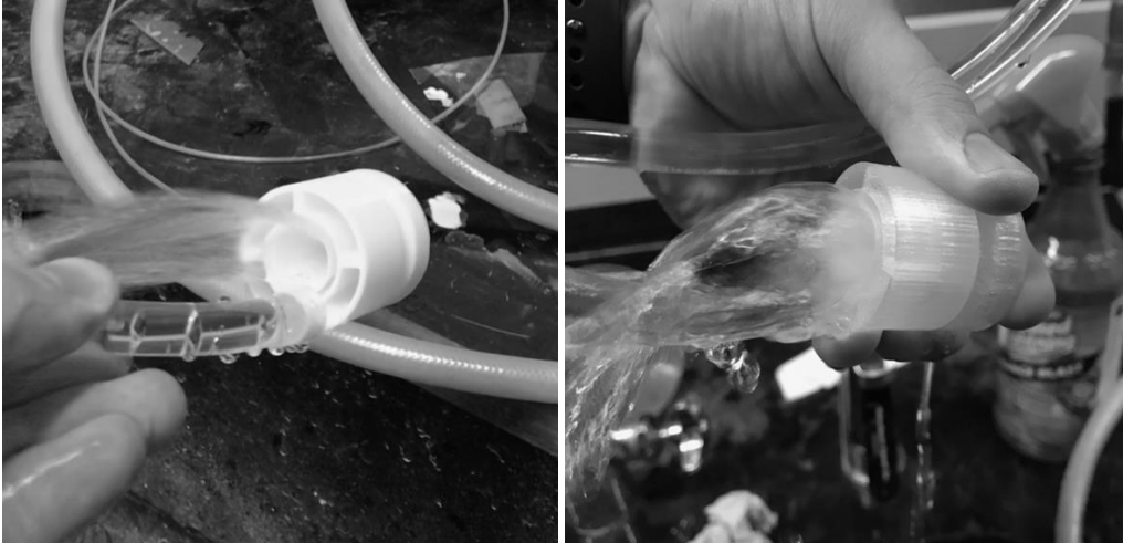
Figure 13: Mark 8 Nozzle Left (Unsuccessful Exit Flow) and Mark 11 Nozzle Right (Successful)
