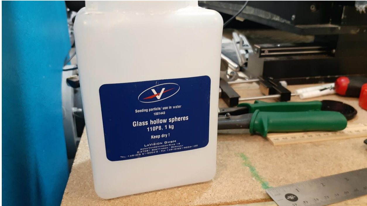
Figure 6: Photo of the LaVision glass seeding particles used.
