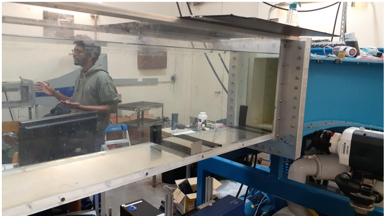
Figure 5: Photo of the flat plate secured to the floor of the water tunnel test section entrance.
