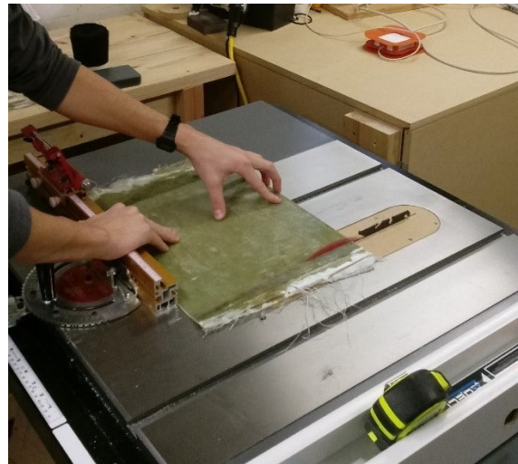
Figure 12. Edges being trimmed from the sheet
