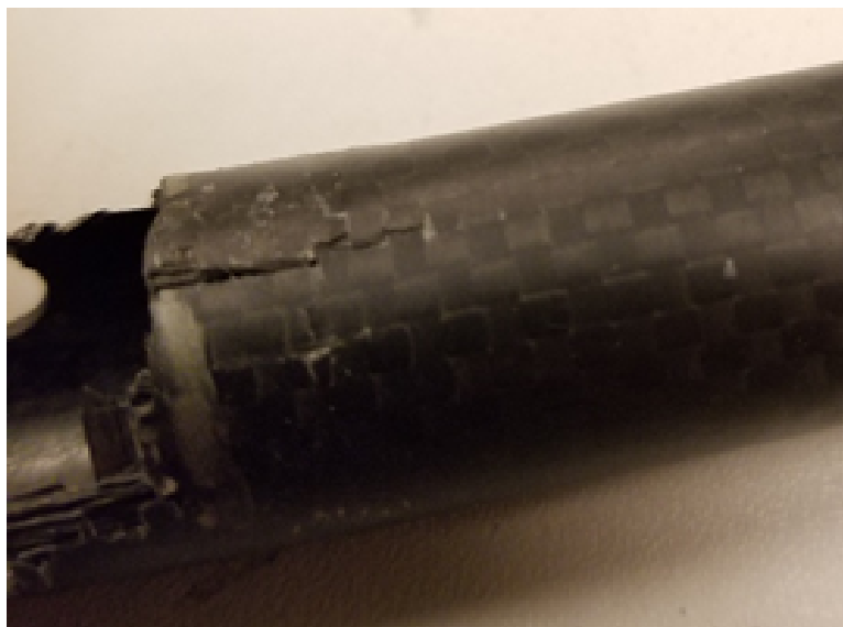
Figure 31. Cracking carbon fiber arm
