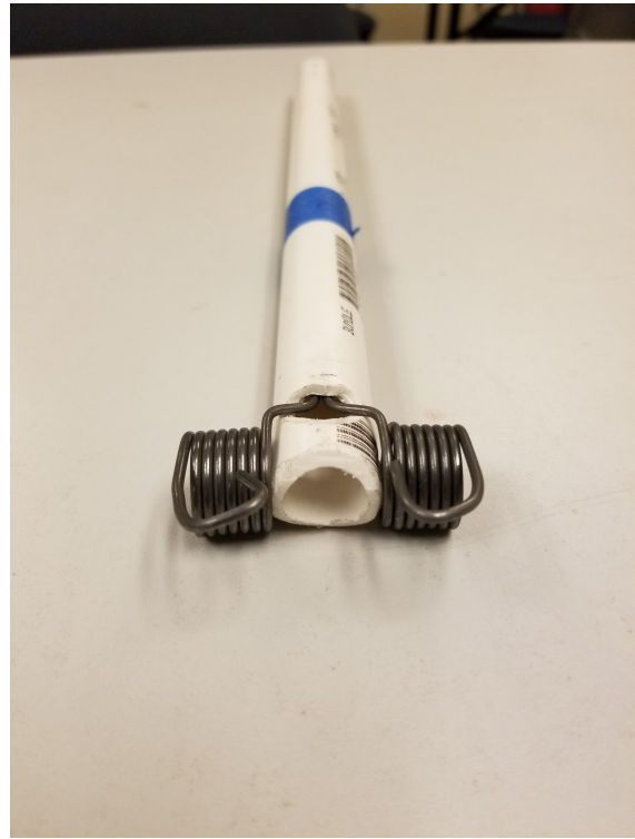
Figure 21. Arm spring system
