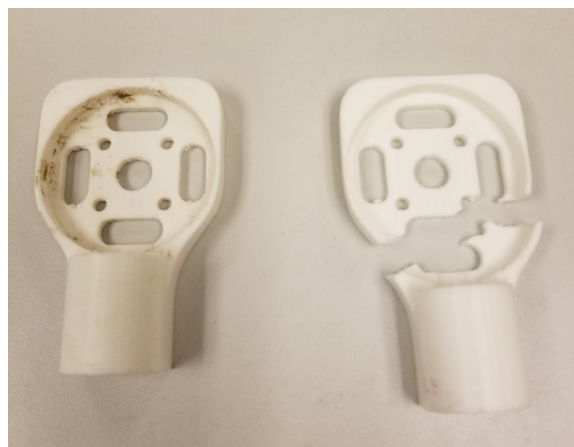
Figure 24. Printed motor mounts
