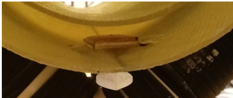
Figure 5. Rail button secured via wood screw, plywood square, and epoxy
