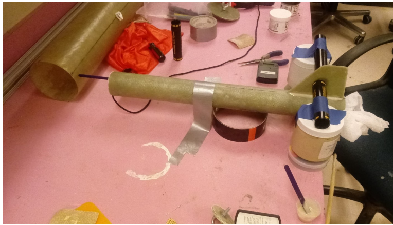
Figure 9. Fin alignment measures
