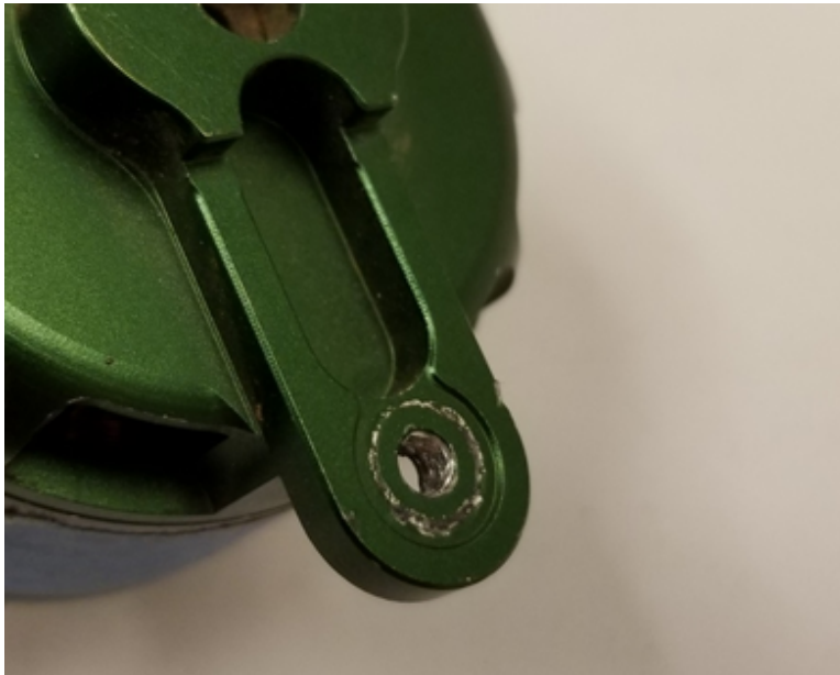
Figure 36. Stripped motor propeller hole
